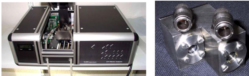
Figure 3-31: Photo of the desktop version of the UV Nitrate analyser (left) and its dual-path length cuvette (right).
