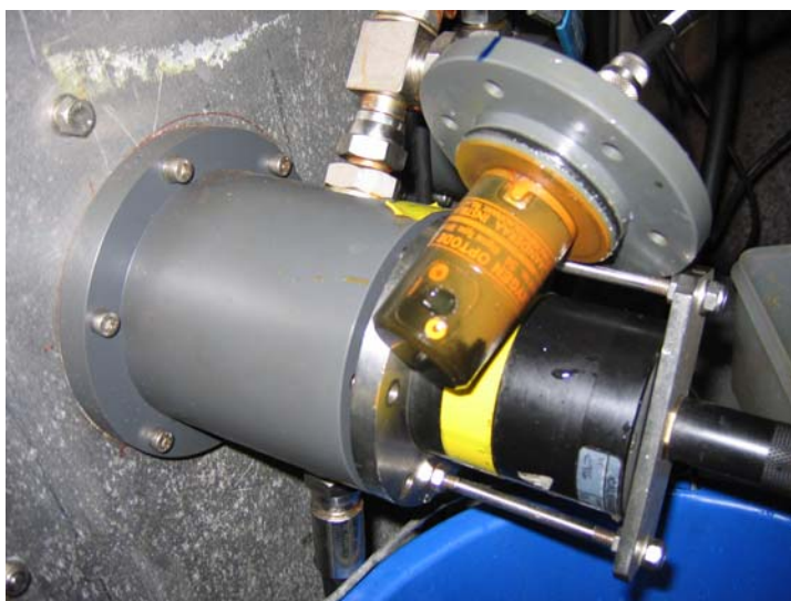
Figure 3-4: Photograph of the Aanderaa Optode removed from its housing for cleaning as installed on the NERC.NOC Ferrybox on “Pride of Bilbao”.
