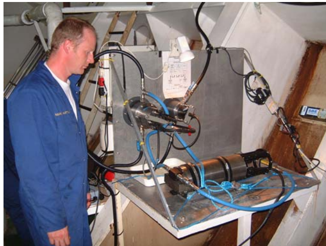
Figure 3-20: Initial test installation of the FRRF in December 2004 as part of the NERC.NOC Ferrybox system on “Pride of Bilbao”.
