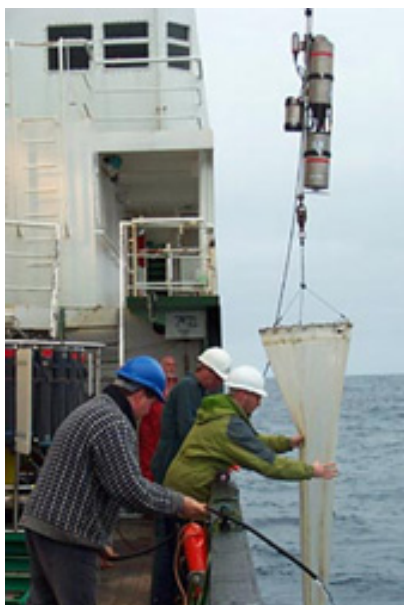
Figure 3-19: Recovery of a normal research deployment of an FRRF in which it is used in conjunction with net sampling of the associated plankton so the taxa present in the water are known and the FRRF response can be correlated with the taxa.
