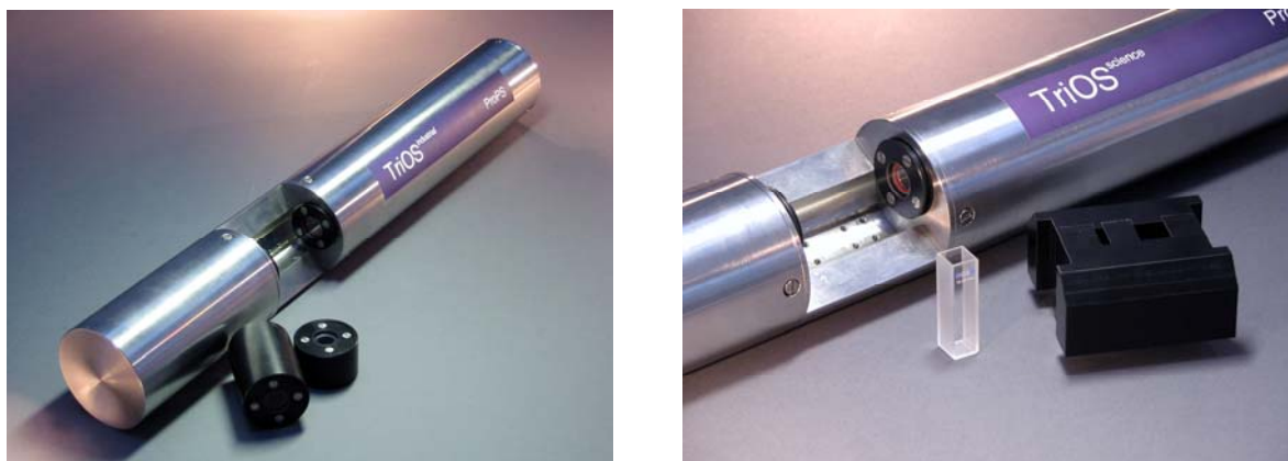
Figure 3-32: Photo of the In situ Analyser "ProPS" (left) with adapters that change the optical wavelengths and a cuvette for lab check (right).
