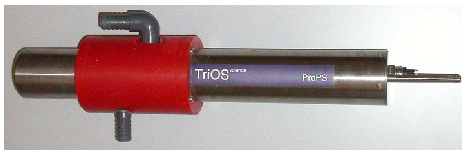
Figure 3-33: The ProPS analyser with customised flow-through unit.
